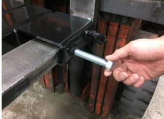
3. Place a C-hook into the end pocket of the T-bar as shown. The C-hook chain grab hook should be facing the fork lift side of the T-bar.
