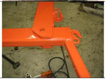
4. Place a disc washer under the C-hook and one above the C-hook. 5. Using a C-hook bolt and spring lock washer, secure the C-hook in the T-bar. Make sure the disc washers are lined up properly so they are not cut by the bolt when it is inserted. 6. Hold the C-hook in place. Place the bolt back into the C-hook and tighten it until the C-hook is snug. Back the bolt up just until the C-hook can rotate. Also take note that the hooks all towards the fork truck when they are installed.
